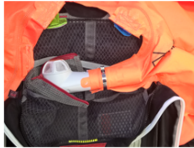
Venturi unit with airbag attachment
